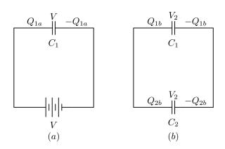
Because the voltage drop across  $C_1$  in situation a is the same as the voltage drop across the battery (V), we have
