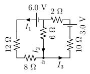
Label the resistors from left to right:  $R_1 = 12 \Omega$ ,  $R_2 = 8 \Omega$ ,  $R_3 = 6 \Omega$ ,  $R_4 = 2 \Omega$ , and  $R_5 = 10 \Omega$ . Label the batteries from left to right:  $V_1 = 6.0 \text{ V}$  and  $V_2 = 3.0 \text{ V}$ . Applying Kirchoff's junction rule to junction *a* we have
