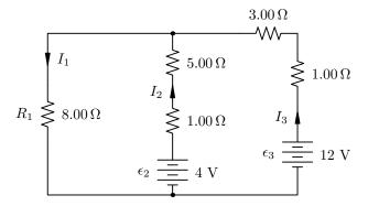
Let  $I_1$  be the current on the left branch (going down),  $I_2$  be the current on the middle branch (going up), and  $I_3$  be the current on the right branch (going up). From Kirchhoff's junction rule, we know.
