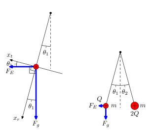
(a) Assuming that the charges are not rotating about each other, the forces on each charge must cancel. The forces on each sphere are gravity  $F_g = mg$ , electrostatic  $F_E = k_e 2Q^2/r^2$ , and tension T. The tension will automatically handle canceling forces in the radial direction, so we need only consider the tangential direction. Let us assume that  $F_E$  is purely in the horizontal direction (see (Note)). Summing the tangential forces on the first sphere
