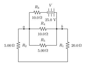
Label the voltage V=25.0 V and the resistances (clockwise from b)  $R_1=20.0\Omega,\,R_2=5.00\Omega,\,R_3=10.0\Omega,\,R_4=10.0\Omega,$  and  $R_5=5.00\Omega.$
