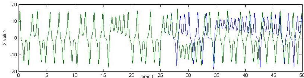
Figure 2 Two numerical solutions of the Lorenz equations showing sensitivity to initial conditions. The  $X$  values, plotted with respect to time, of two trajectories whose initial positions differ by one one-hundred-billionth in the  $Z$  direction. These two trajectories seem identical until around  $t = 27.5$ , at which point they completely separate forever.
