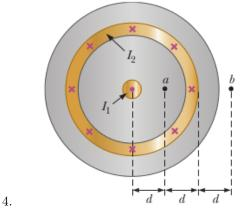
Behold a cross-section of Coaxial cable above. The center conductor is surrounded by a rubber layer, an outer conductor, and another rubber layer. In a particular application, the current in the inner conductor is  $I_1 = 1.00$  A out of the page and the current in the outer conductor is  $I_2 = 3.00$  A into the page. Assuming the distance d = 1.00 mm, determine the magnitude and direction of the magnetic field at (a) point a and (b) point b. *Hint: Use Ampere's Law*.
