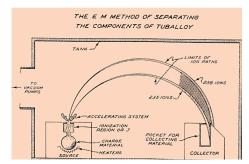
However, it isn't efficient enough for industrial level production; a high-end mass spectrometer could, on the other hand, use this effect to measure how much of a given uranium sample is the weapons-grade 235 verses the more common 238.
