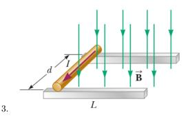
A rod of mass 0.720 kg and radius 6.00 cm rests on two parallel rails (see figure) that are d = 12.0 cm apart and L = 45.0 cm long. The rod carries a current of I = 48.0 A in the direction shown and rolls along the rails without slipping. A uniform magnetic field of magnitude 0.240 T is directed perpendicular to the rod and the rails. If it starts from rest, what is the speed of the rod as it leaves the rails?
