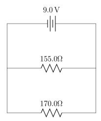
We know that the current passing through the separate branches will not be the same unless the resistor is the same, so that we need to apply the junction rule:
