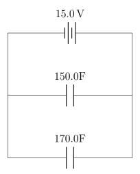
The voltage drop across each capacitor is the same, and so the total charge on both capacitors is
