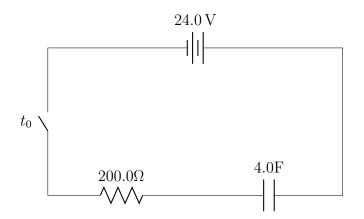
1. Find the charge, as a function of time, on the capacitor for the above circuit when the switch is closed. What is the value for each at 3 seconds in?
