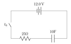
The switch is shown to be open, and this means the circuit is not activated—no current flows. Now the switch is activated:
