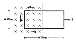
15. In the figure above we see a single rectangular loop of wire with given dimensions situated inside a region of uniform magnetic field of 0.550 T. The total resistance of the loop is 0.230  $\Omega$ . Calculate the force required to pull the loop from the field (to the right) at a constant velocity of 3.40 m/s. Ignore gravity.
