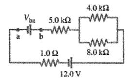
17. The current through the 4.0 k $\Omega$  resistor in the above circuit is 3.50 mA. What is the terminal voltage  $V_{ba}$  of the unknown battery  $V_{ba}$ ? Assume that the current direction is to the right. Bonus: What if we were to assume the current direction is to the left? Hint: Use the loop rule (also known as Kirchhoff's rule).
