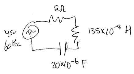
$X_{L} = \omega L = 2\pi (60) 135 \times 10^{-3} H = 50.9 \text{ T}$   $X_{C} = \omega C = \frac{1}{2\pi (60)} (20 \times 10^{-6} \text{ P}) = 132.63$   $Z = \sqrt{R^{2} + (X_{L} - X_{L}^{2})}$   $= \sqrt{2^{2} + (3248) 50.9 - 132.63}$
