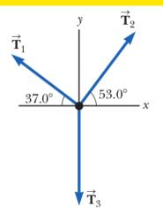
Now draw the free body diagram for the intersection of the three cables.
