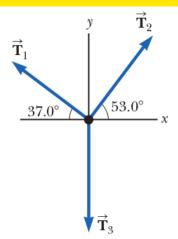
Now draw the free body diagram for the intersection of the three cables.
