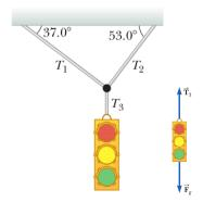
First, draw the free body of the light with only the cable attached to it.
