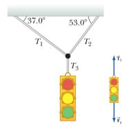
First, draw the free body of the light with only the cable attached to it.
