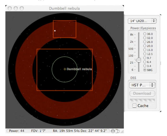
Equinox 6 can display an SBIG outline in the Scope View window if it knows what camera is being used. Eyepiece 10 is reserved for SBIG outline use in this case. The SBIG outline can be used to help locate guide stars, centering faint objects and determining what camera angle is required to put a guide star into the guide chip image. The guide chip outline will rotate to the current camera angle if the autoguide calibration has been done.
