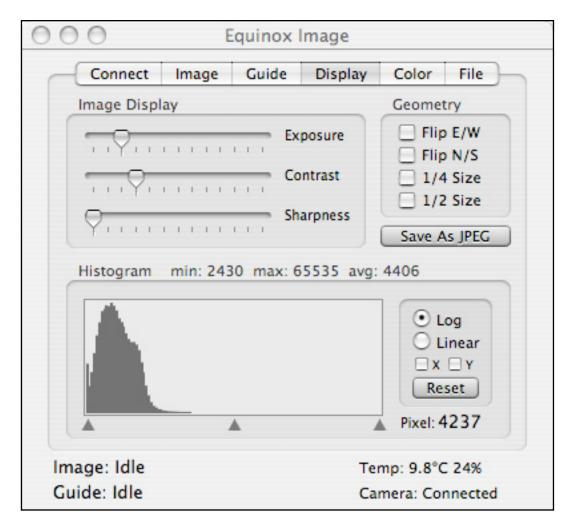
The controls in the Display tab give you several different ways to manipulate the image. *Note that none of these controls change the raw image saved to disk.* You can alter the effective exposure, contrast and sharpness with slider controls, flip the image and reduce the size (so you can see the entire image within the window). If you select both the 1/4 and 1/2 boxes the image will actually be scaled up 2X.
