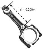
$$f = \frac{100 \text{ swings}}{120 \text{ s}} = \frac{5}{6} \text{ Hz} \quad \left[ W = 2\pi f = \frac{5\pi}{3} \text{ rad/s} \right]$$
