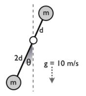
Consider the lopsided pendulum pictured above. Assume it is free to rotate in the plane of the page but otherwise fixed. Each sphere has uniform density and mass m. Neglect the mass of the rod and assume  $g = 10 m/s^2$ , m = 5 Kg, and d = 1 m.
