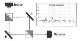
If the second beam splitter is tuned so that only the beam coinciding with mirror B is directed to the detector then only prominent peak in the Power Spectrum is the frequency of that mirror.
