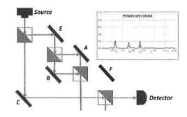
And finally, if the path from mirror C is completely blocked then we arrive at no frequencies in the power spectrum of the detector signal. This is something of a sanity check as we can verify there are no obvious leaks in the system.
