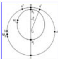
FIGURE 8.3.1.- A planet at  $O$  has two orbiting satellites, one of small mass ( $M_2$ ) moving in a circular orbit and one of negligible mass ( $M_1$ ) moving in an elliptic orbit. The orbital inclinations are zero and the
