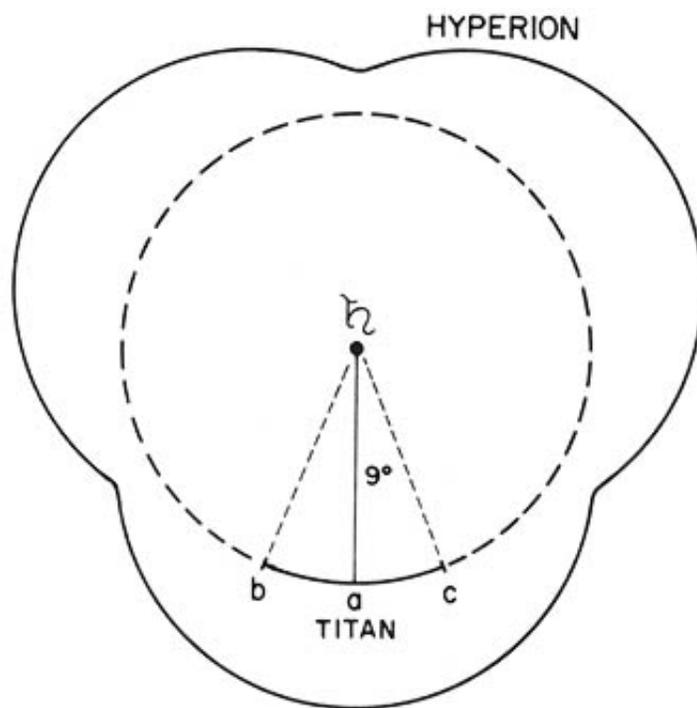
FIGURE 8.5.5.- The orbital pattern for the  $4/3$  resonance of Titan-Hyperion in the Saturnian satellite system. Titan librates with an amplitude of  $9^\circ$  about the equilibrium position at **a**. The orbit of Hyperion is strongly perturbed by Titan.
